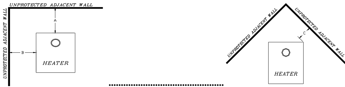
FIGURE 1.3 Clearances to combustible materials
