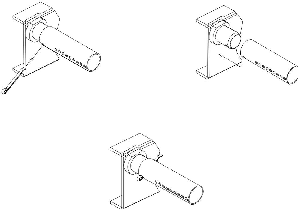
**Figure 4.3 – Secondary Air Tube replacement**
