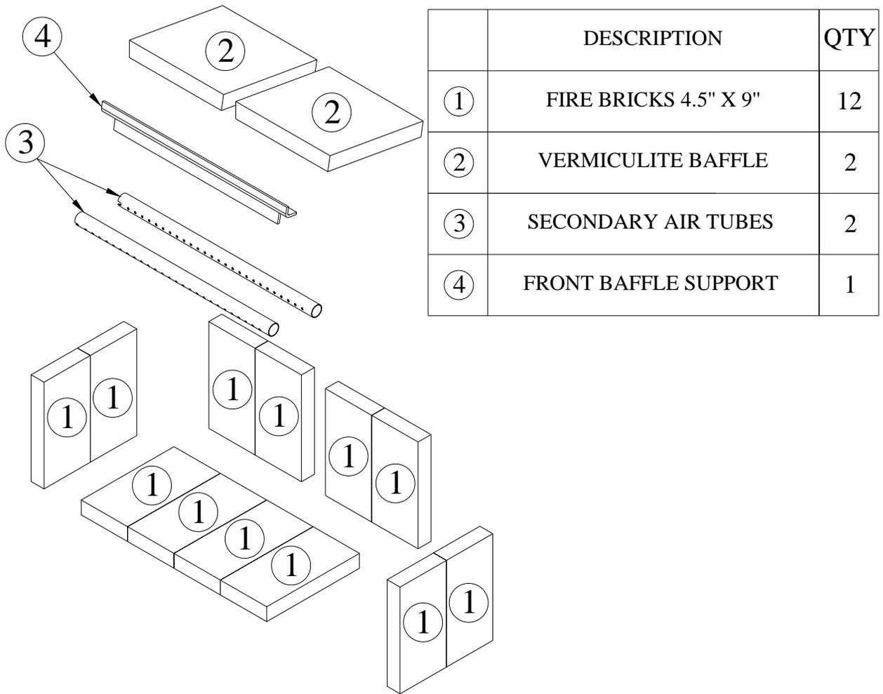
**Figure 4.2 – Firebrick layout for Osburn 1100 Insert model**
