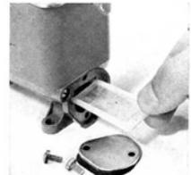
4. Surround area with oil absorbent material. Place a V-shape funnel under filter cover, remove cover screws, and drain into pan. Remove filter. Clean filter in fresh heating oil, kerosene, or hot water. If you use hot water, thoroughly dry filter before installing.
