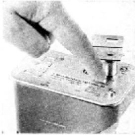
2. Set oil control knob to highest position and tap thermostat pin. This will help remove a slight accumulation of dirt in the metering stems slit. CLOSE oil control.
