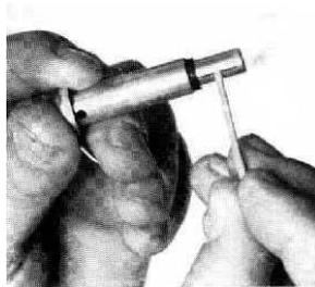
4. Remove metering stem and clean slit. Cleaning should be done with a soft, non-metallic instrument. The slit must not be enlarged.
